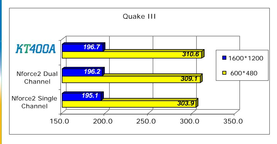
KT400A Test Set Up: KT400A Reference Board + AMD Athlon XP 2800+, 512MB Winbond DDR333, Maxtor DX740X-6L 40GBHDD, Windows® XP
